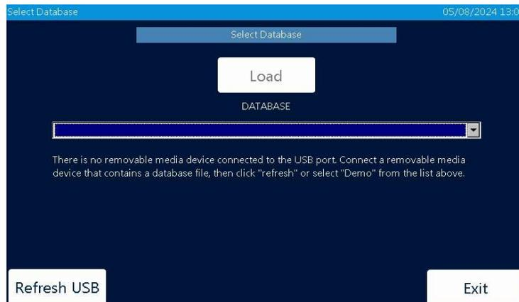
From the dropdown menu choose the database you have loaded into the AccuFIT 9000 Internal Memory and tap “Load”
