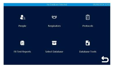
At this point you should remove the USB thumb drive from the AccuFIT 9000 device, as you want to be sure that you are addressing the database that has been transferred to the AccuFIT 9000 Internal memory rather than the database on the USB thumb drive. Tap "Select Database".
