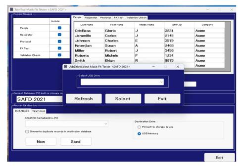
Using the dropdown menu in the new pop-up window highlight the correct thumb drive and tap "Exit" in the pop-up window.
