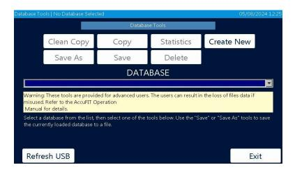
Highlight the database you want to transfer to the AccuFIT 9000 Device from the dropdown menu. If the database you want to transfer does not appear, tap "Refresh USB". The database will then appear in the dropdown box, but will not be loaded into the device's active memory. Tap the "Copy" command box in the top half of the screen if you want to copy the entire database
