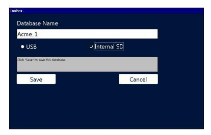
The Copy Screen appears and provides the choice of copying to "USB" (thumb drive) or "Internal SD" (the device's internal memory). Select "Internal SD". At this point you are given the opportunity to rename the database before saving to the internal memory by using the pop-up touchpad. Once you have renamed the database (or not, if you choose to accept the assigned name) tap "Save".
